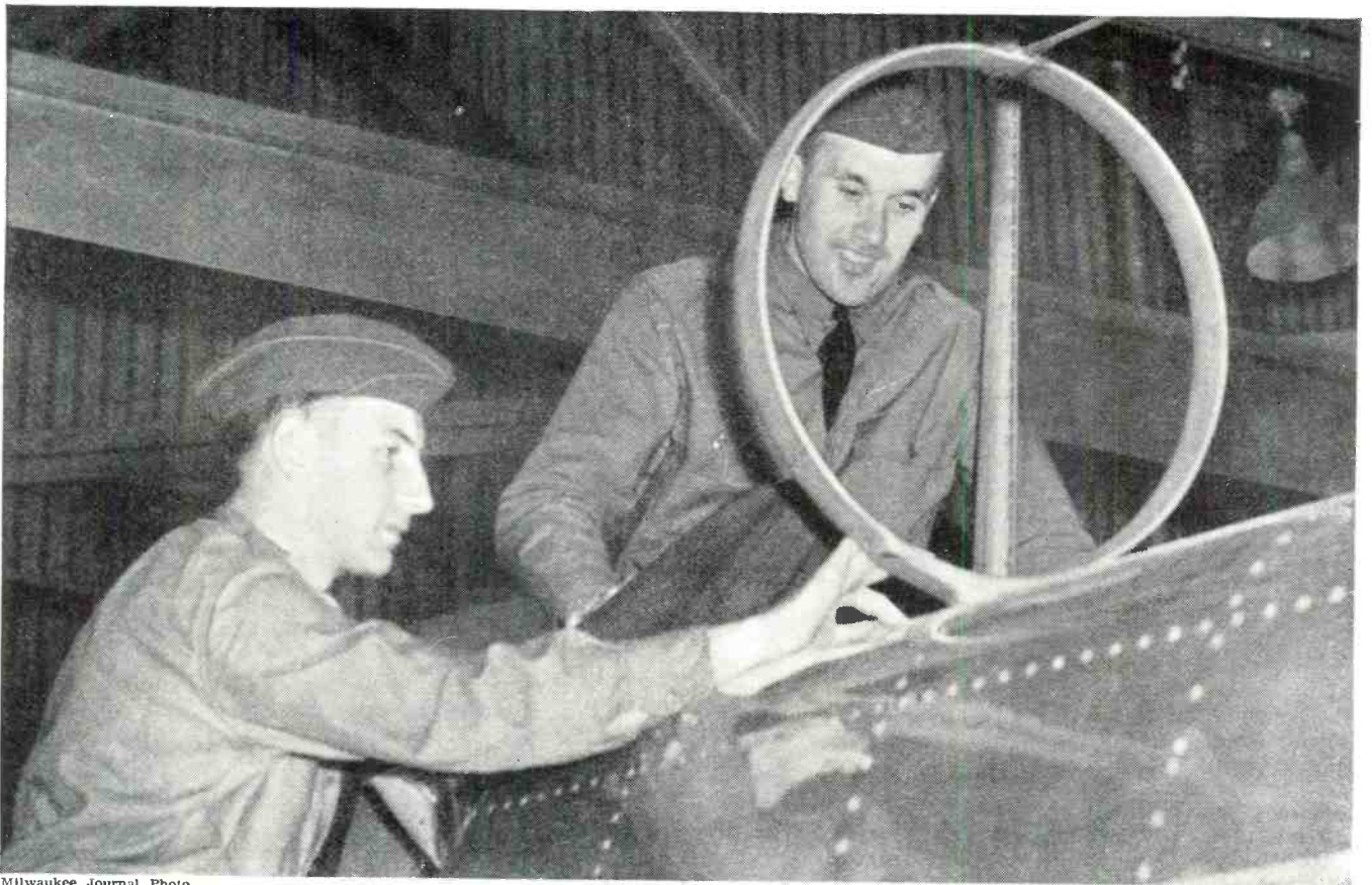
Flying cadets learn to be communications officers. A directional loop antenna is examined by two students.
