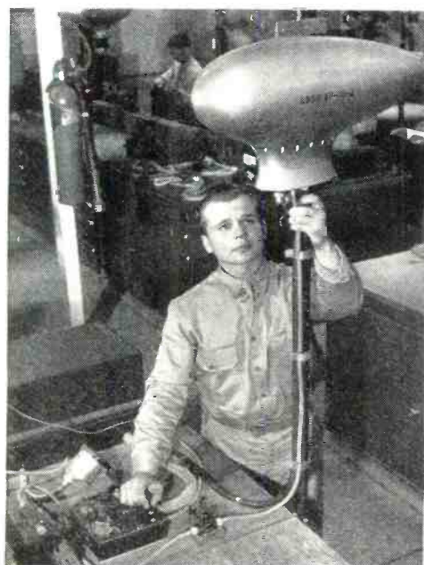
Student operates shielded loop antenna. It resembles a miniature blimp.
