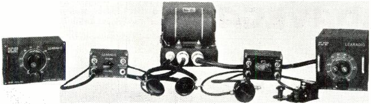
Complete UHF components set up for test before installation in the aircraft. Receiver covers 21-29 mc. range.
