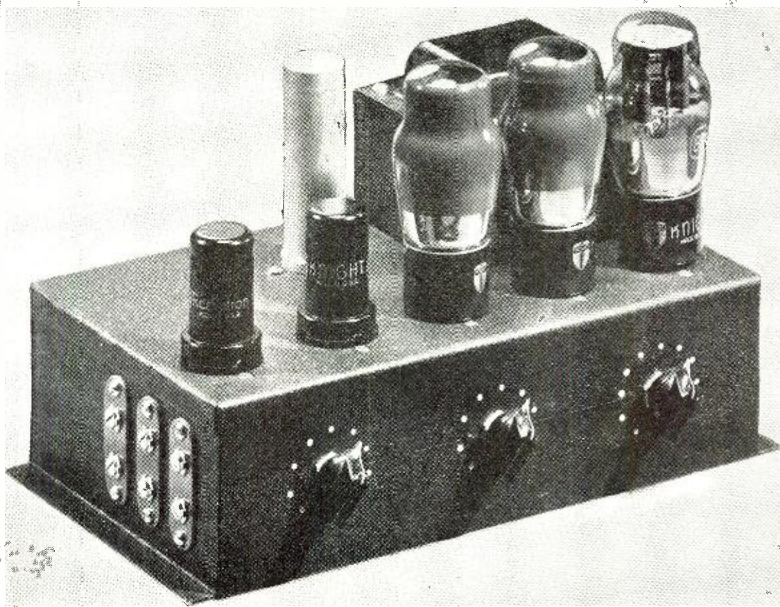
Connections to the amplifier are made at the terminals mounted on the side of the chassis.
